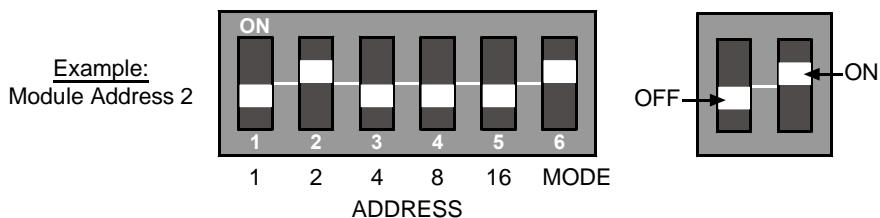
Figure 29: Command Center DIP Switch Orientation
